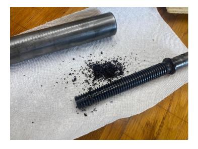
Fortunately, that is dirty, oil-soaked wood chips and not metal fragments. However, the screw effectively had no lubrication. Cleaning is as simple as removing the handle and sliding the quill/screw assembly out. Then take those apart and thoroughly clean everything. I use WD-40 and a toothbrush. You can lubricate either with a light oil or grease. I am currently using a spray white grease. It moves smoothly now even when pushing a 1 ½ big into end grain.
