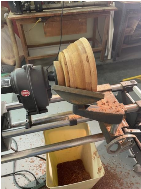
Outside turning set-up on a Shopsmith Speed Reducer and Standard Tool Rest
