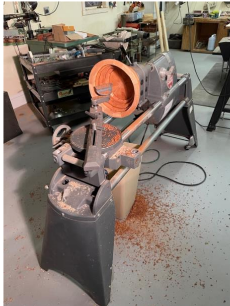
Inside turning set-up on a Shopsmith Speed Reducer and Universal Tool Rest
