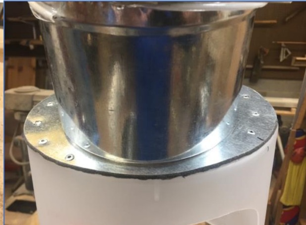
Photo 4-Top of hood showing the 6" Air Tight Air Take Off with a tacky gasket. The flange was cut to match the waste can bottom and pop riveted. The
