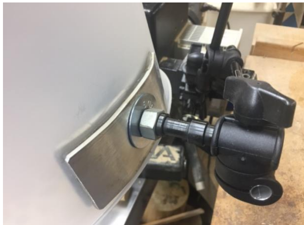
Photo 3- Aluminum outside bracket and arm-Note- the large nut is used only for a spacer
