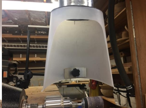
Photo 6- Front of the dust hood showing the cut out of the wastebasket and the knob tightening the articulation arm and the formed bracket
