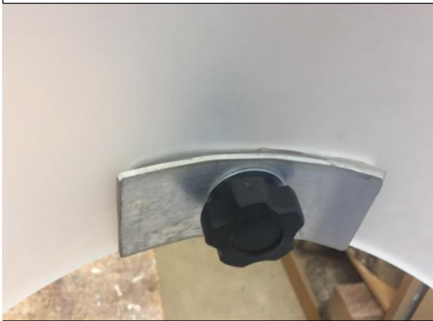
Photo 7- Close up the tightening knob and bracket with the double stick tape.
