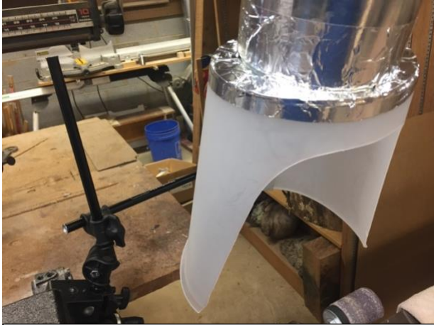
Photo-9- Completed hood with aluminum tap sealing the joints.
