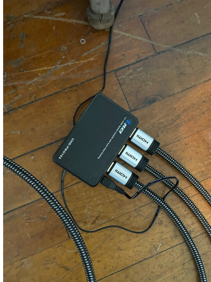
Splitter with Input from PC and outputs to the wall connectors
