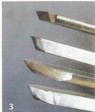
3 The bevels on my scrapers start at about 45° on the nose, becoming near vertical on the side.
