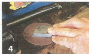
4 The bevels on my scrapers start at about 45° on the nose, becoming near vertical on the side.
