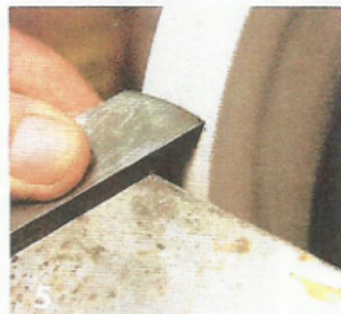
The bevels on my scrapers start at about 45° on the nose, becoming near vertical on the side.
