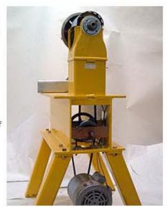
underneath the bed on a jack shaft. The jack shaft also has a three-step pulley that connects by belt to a three-step pulley on the headstock. Manually moving the belt on the stepped pulleys changes the speed.
