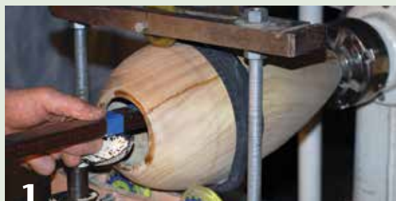
1 A heavy boring bar is positioned to cut deep inside the re-glued wing vessel.
