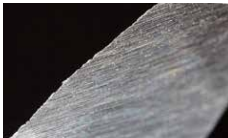
The edge of a gouge sharpened on my dry grinder
