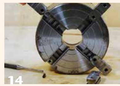
14 Reinstall the jaw slides in sequential order.
