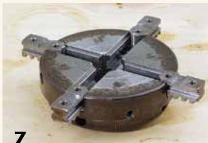
7 The jaw slides are ready to be removed by hand.
