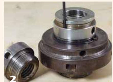
2 Inspect your chuck for locking grub screws and back them out to avoid thread damage.
