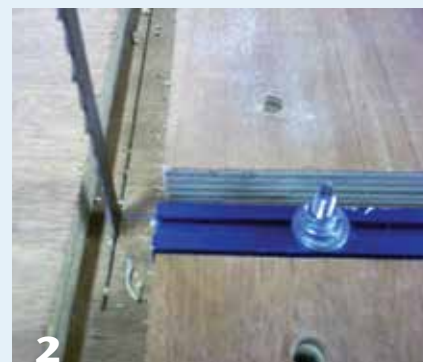
2 The track holding the pivot pin. Move the pin back and forth to cut blanks of different diameters.
