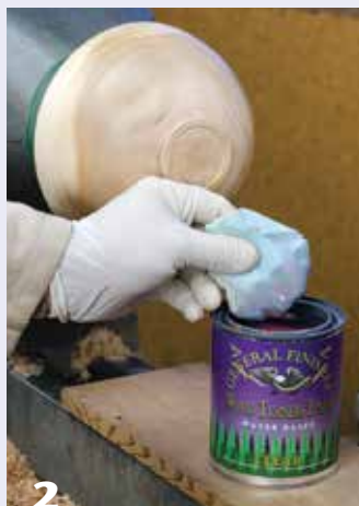
2 A shop towel tucked in a nylon footie is General Finishes' recommended applicator for Wood Turners Finish.
