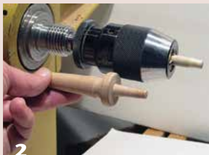
2 A 3/8" (10mm) dowel inserted into a Jacobs chuck serves as a mandrel to hold the turning blank.
