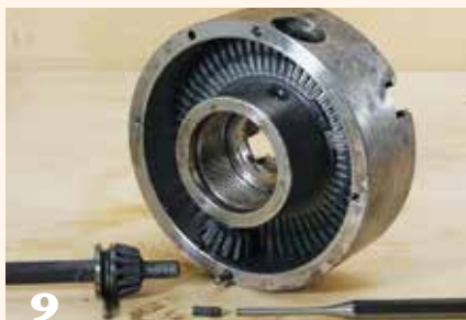
9 Exposed inner workings of geared chuck. Note the small grub screws that secure the pinion dowels.
