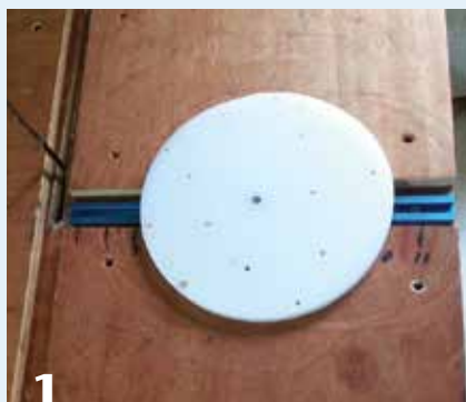
1 The jig has a runner to fit in the saw's miter slot. A disc made from a cutting board fits over a bolt in a track perpendicular to the blade.
