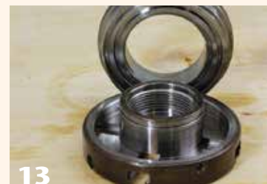
13 Reassembly starts with the scroll ring (lever chuck) or gears.
