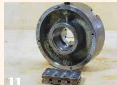
11 A light coat of grease, light oil, or dry lubricant keeps wear to a minimum.
