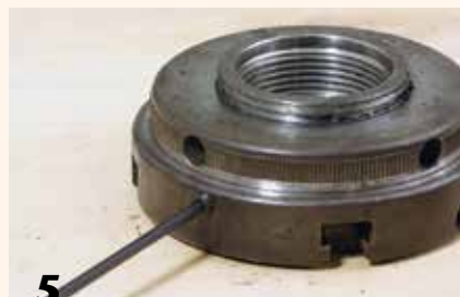
5 Check for a grub screw that regulates the scroll action and remove it if your chuck has one.
