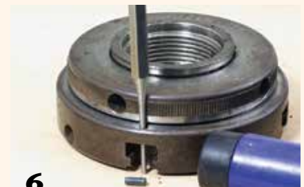
6 Removing the stop pins that prevent the jaws from backing out of the chuck body.
