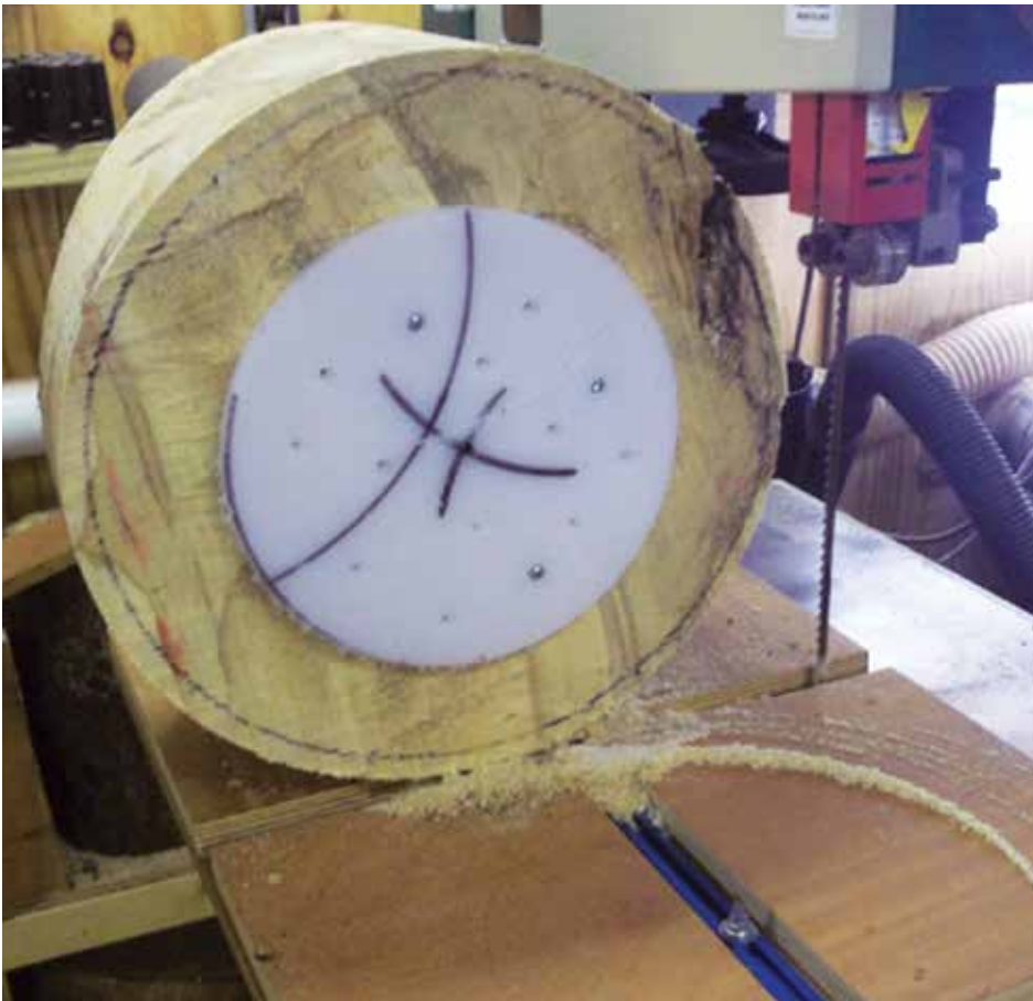
Plywood, some simple hardware, a pen bushing, and a cutting board combine to make a safe, easy-to-use jig for cutting bowl blanks.
