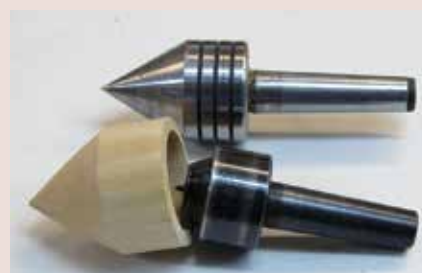
4 If you do not have a 60-degree cone center, turn one to fit over your existing live center.
