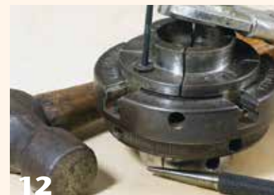
12 Carefully directed blows can clench a deformed screw head around an Allen wrench.
