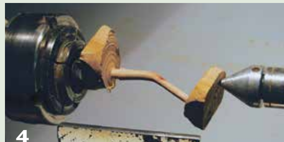
4 Off-center turning of a toe. The tenon cut for joining the toe to the foot pad is visible on the left where the toe joins the blank.
