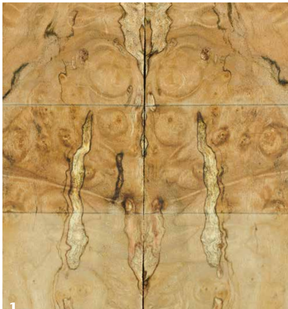
1 A spalted maple sample board contrasts thinned tung oil (middle) with General Finishes Wood Turners Finish (top), and Varathane Polyurethane Satin (bottom).
