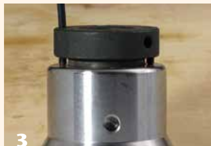
3 A Taper-Lock spindle adaptor is removed by alternately tightening hex screws against the chuck body.
