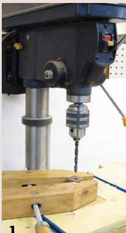
1 A wooden parallel clamp with a pair of opposing notches cut out will firmly hold turning blanks for drilling.
