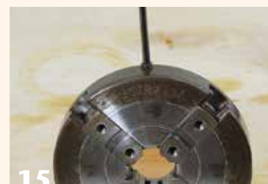
15 Setting the washer and grub screw to establish resistance in the scroll mechanism.
