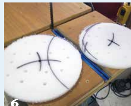
6 Drill counterbored holes in the discs to serve as mounting holes for the wood blank.
