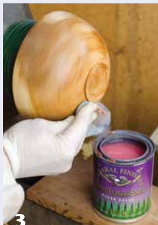
3 The dampened applicator is held against the rotating piece. The objective is to quickly apply a thin coat over the entire piece before the finish begins to cure and become gummy.
