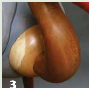
3 The holly breast piece and the lower section of the sycamore neck are both turned.
