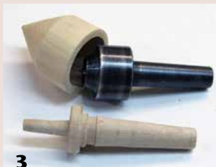
3 If you do not have a Jacobs chuck, turn a mandrel with a Morse taper to fit your lathe.
