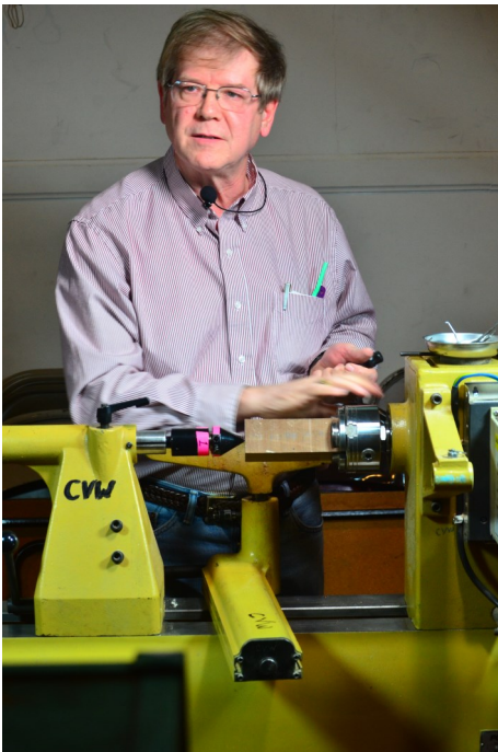
Ray with the blank mounted in the chuck ready to begin turning.
