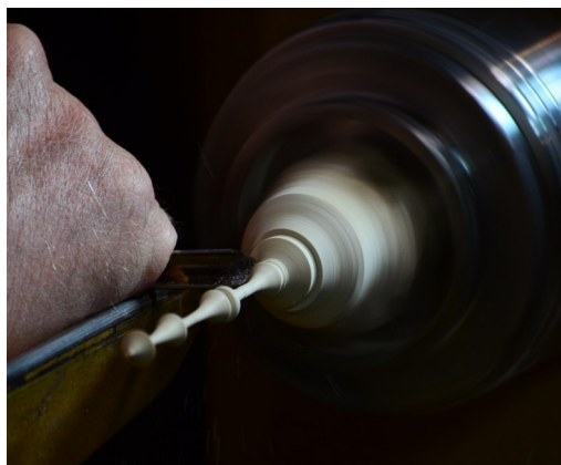
The bottom finial is well under way. Photo by David Rhodes
