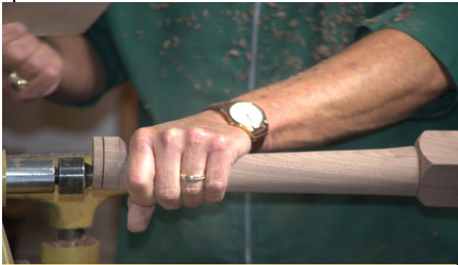
Remounting on new axis to turn foot pad Photo by David Rhodes
