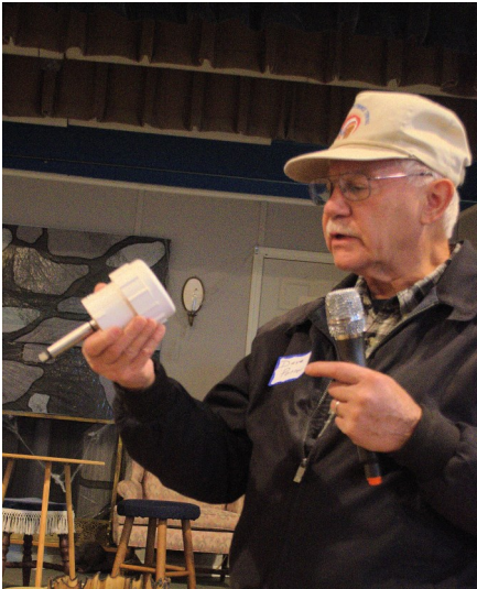
Dave Potter shows the chuck he made from PVC for his Singapore sphere. Photo by David Rhodes
