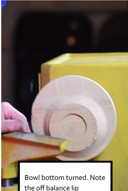
Air cutting the bowl lip Note the new recess has been cut for the second axis
