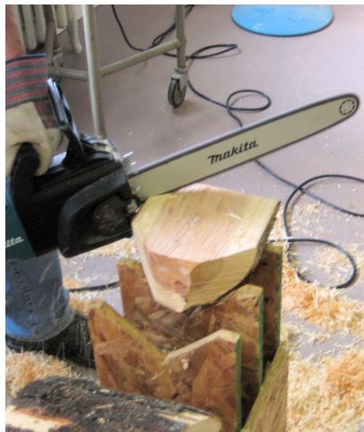
Left: Don's jig in use to trim a green wood blank for turning. Photo by Dennis Hippen
