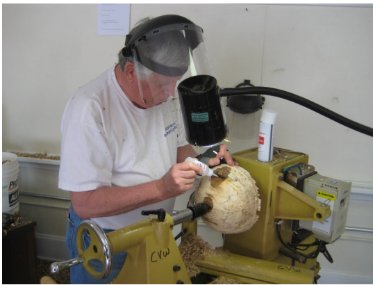
Jim Guynn applies a bit of CA glue to the piece he is turning
