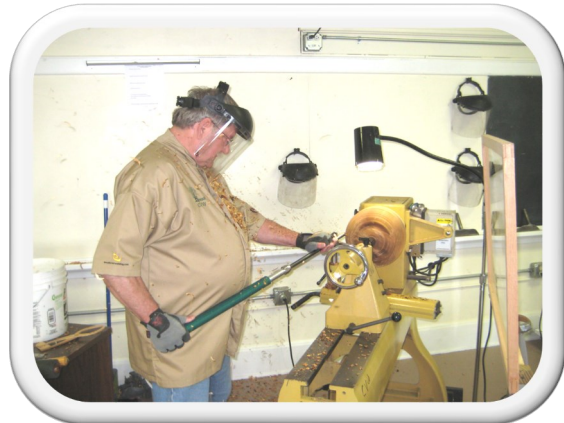
Dennis hard at work turning the bowl. Note the safety emphasis: good lighting, face shield, and Plexiglas safety shield in front of the lathe to protect the audience.
