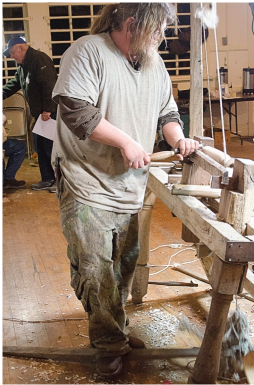
Left: Turning a baby rattle with the lathe at full foot power speed. Photo by David Rhodes
