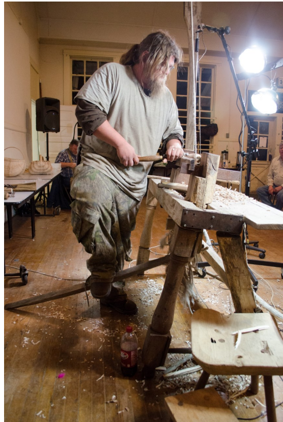
Below Right: Nathan and his lathe at work.. Note Nathan's right foot on the treadle supplying the power for the lathe.. Photo by David Rhodes
