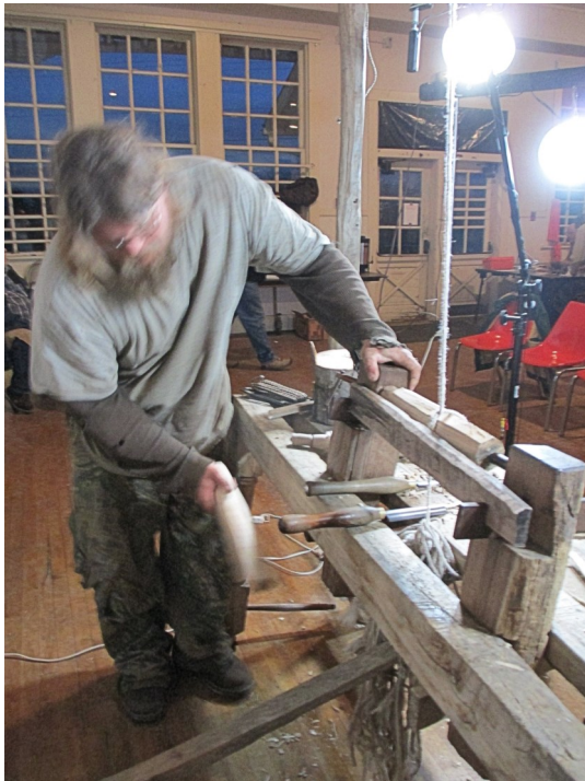
Left: Nathan tightens the headstock Above: Goblets turned by Nathan on his treadle lathe.
