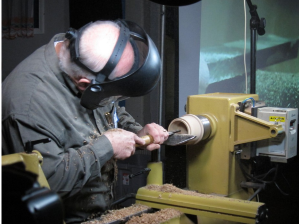
Left: Hollowing the base and, right: marking the base diameter on the lid Photos by Fred Williamson.
