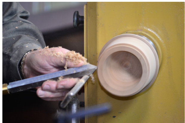
Above left: Roger shows a pair of finished boxes. When making a box, Roger begins with the base making the top last. Here he is preparing a tenon on the base for the lid. Photos by David Rhodes
