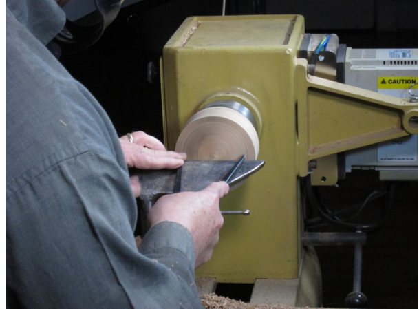
Left: Hollowing the base and, right: marking the base diameter on the lid Photos by Fred Williamson.
