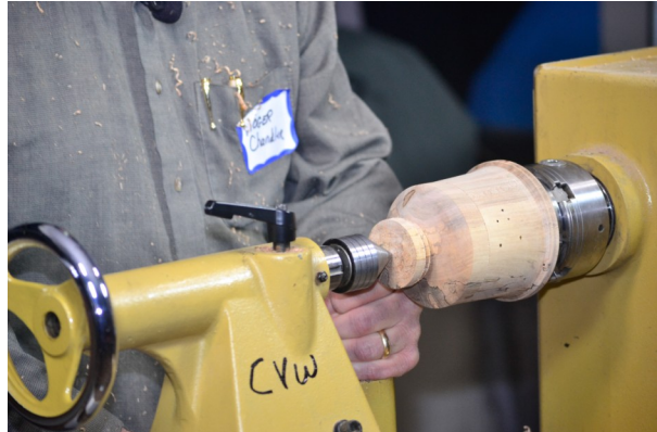
Left: Shaping the lid. Requires good tool control .Right: After reversing lid/base in chuck, turning the knob. Photos by David Rhodes.
