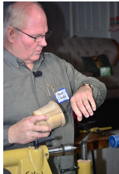
Left: Roger has reverse chucked the base using the Rubber Chucky in preparation for finishing the bottom
