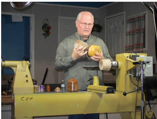
Above left: Roger shows a pair of finished boxes. When making a box, Roger begins with the base making the top last. Here he is preparing a tenon on the base for the lid. Photos by David Rhodes
