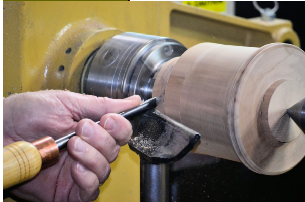
Left: Shaping the lid. Requires good tool control .Right: After reversing lid/base in chuck, turning the knob. Photos by David Rhodes.
