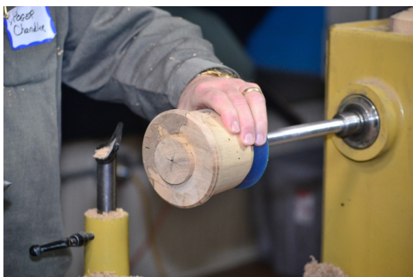
Left: Roger has reverse chucked the base using the Rubber Chucky in preparation for finishing the bottom
