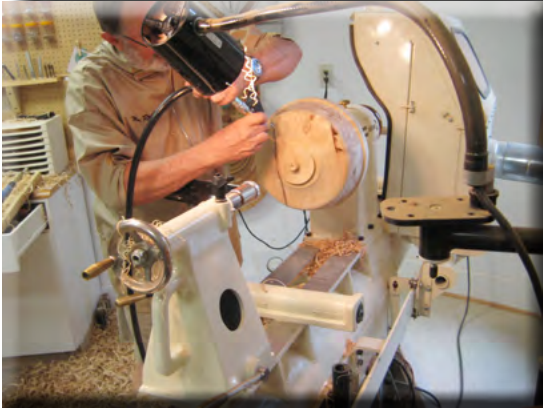
Marc cleaning out bark inclusion & the deep crack with air compressor.
