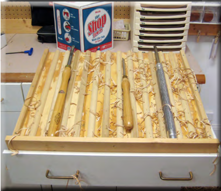
Note the handy tool parking caddy near lathe resting on an open drawer.
