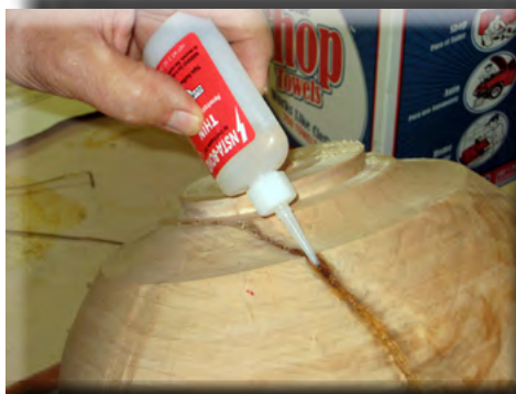
Place some thin CA at bottom of crack to glue hard to reach areas.
