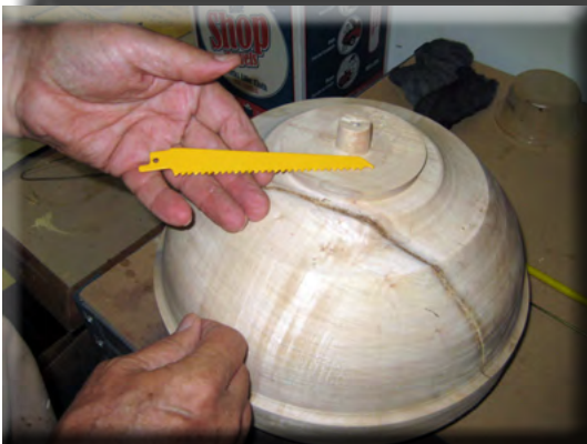
A Sawzall blade is an ideal tool to help clean out the crack.
