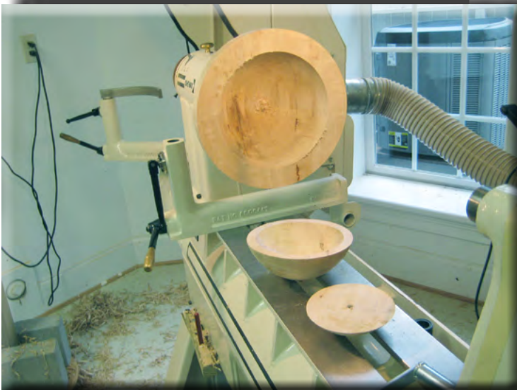
Marc used his Oneway coring system to gain 3 bowl blanks from the single blank.
