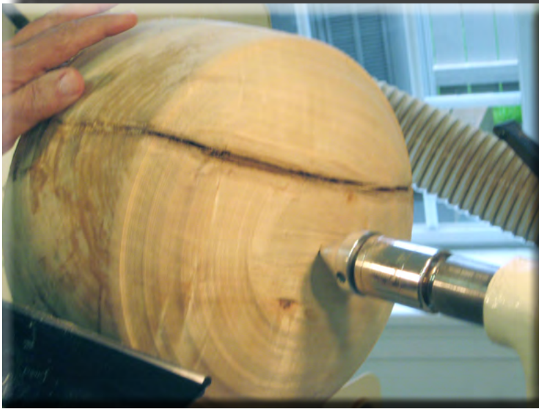
Green Ambrosia maple 14" bowl blank from Waynesboro. It has a deep crack with some bark inclusions.
