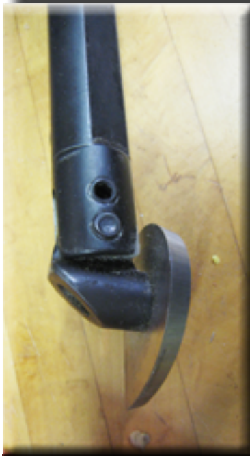
The Kelton adjustable scraper looks like it would be a highly versatile and effective tool ( http://www.kelton.co.nz/Kelton%20Multi-Axis%20Scraper.html )
