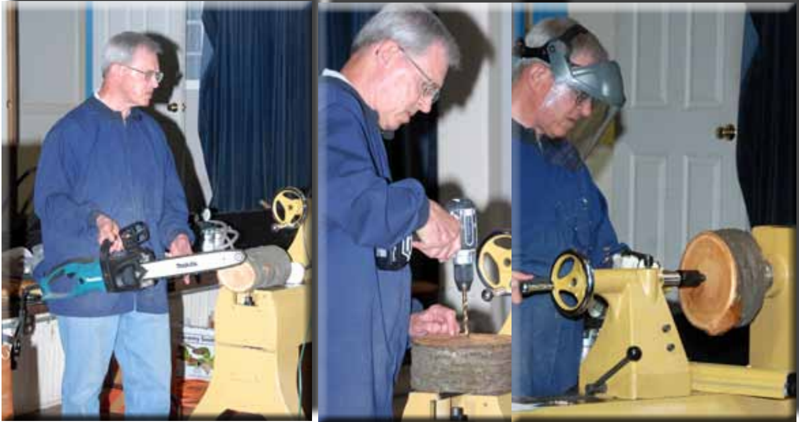
Don used a chain saw to trim the ends of his small log and to cut it to length for the lathe. He then drilled a 3/8" hole. He used a screw chuck adapter in his 4-jaw chuck on which to mount the wood.
