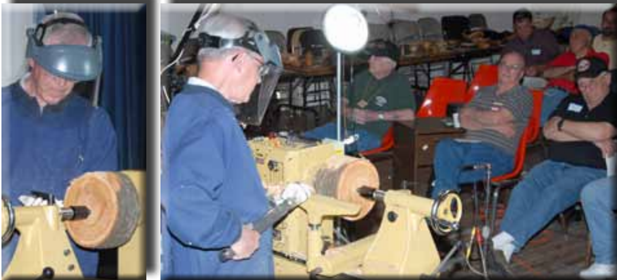
Don used a chain saw to trim the ends of his small log and to cut it to length for the lathe. He then drilled a 3/8" hole. He used a screw chuck adapter in his 4-jaw chuck on which to mount the wood.
