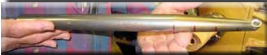
Among the many carbide-tipped turning tools on the market these days, the Eliminator Hollowing Tool has been around for several years. The 90 degree flats milled on the bottom provide an ideal angle for shearing cuts and add stability. Barbara has two sizes of this tool ad like them.
