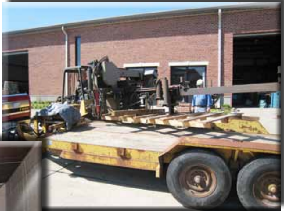
Large metal-cutting band saw with auto-feed and pneumatic vises.
