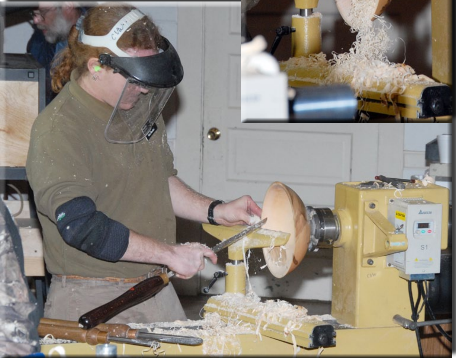
Using a bowl gouge angled up and cutting with the side of the fingernail grind, Nate makes a smooth finishing cut on the inside of the bowl. (Note the fine shavings) He learned this technique from our own Fred Williamson.
