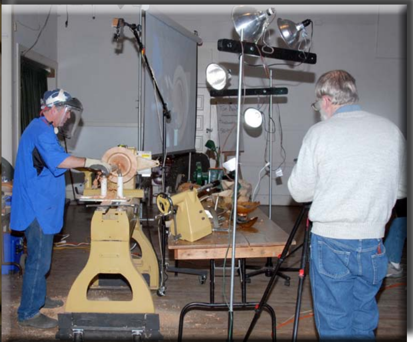
Muscle is required to force the carbide cutter through the wood. Frequent chip clearing is required.
