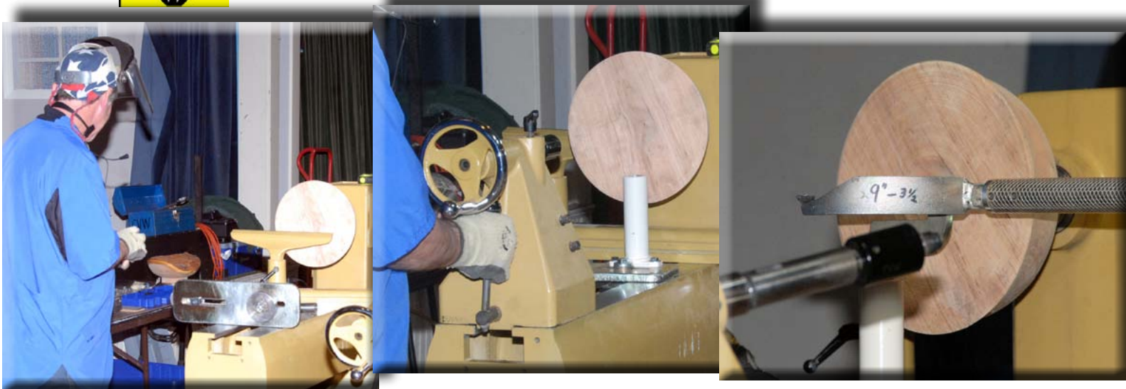
Kirk had made a steel plate on which to mount the components of the coring system.
