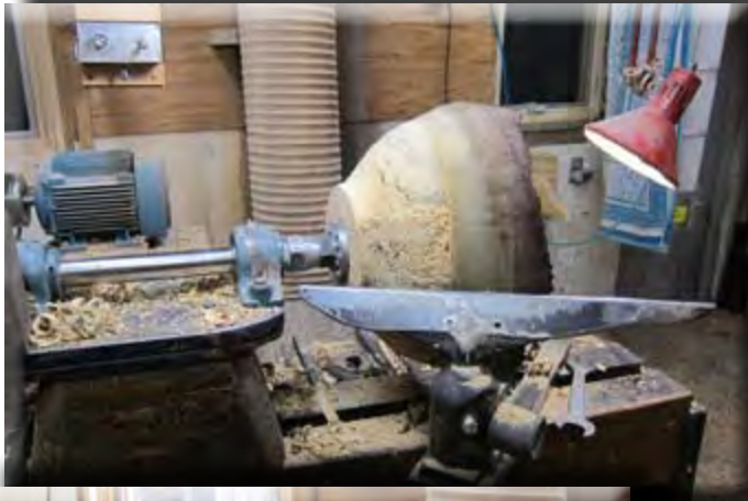
Fred is using a custom, longer cutter to core a piece of the Montecello yellow poplar.
