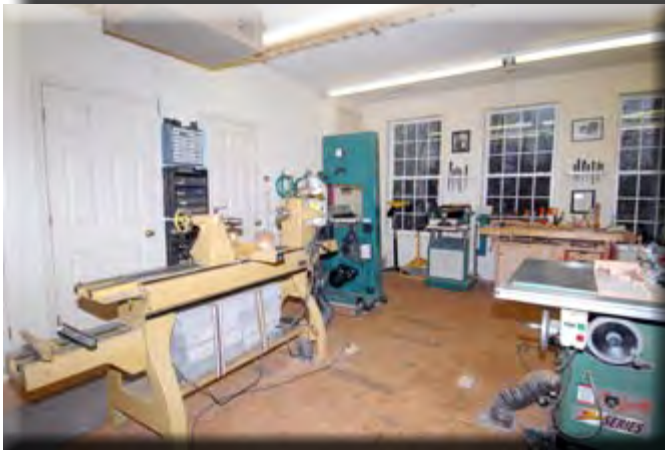
Hal's PowerMatic 3520B is located near his dust collector (behind one of the doors) and next to the band saw; characteristic of a good wood turner. Note the cement blocks under the 3520 to add weight and stability.
