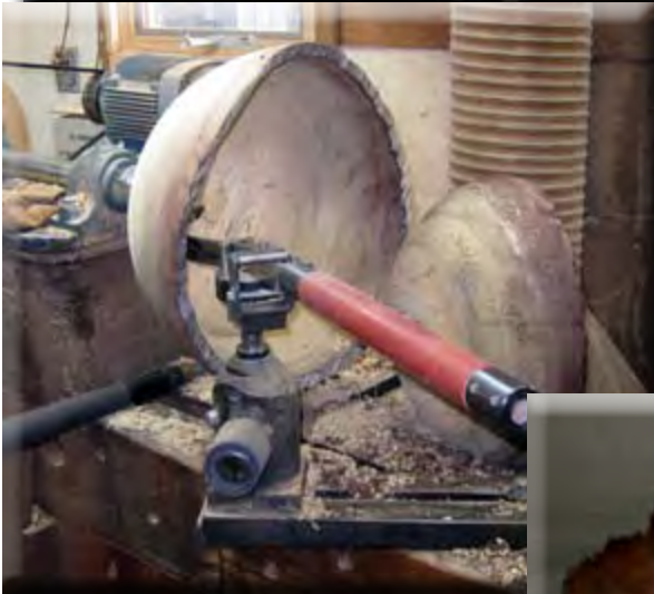
Fred is using a custom, longer cutter to core a piece of the Montecello yellow poplar.
