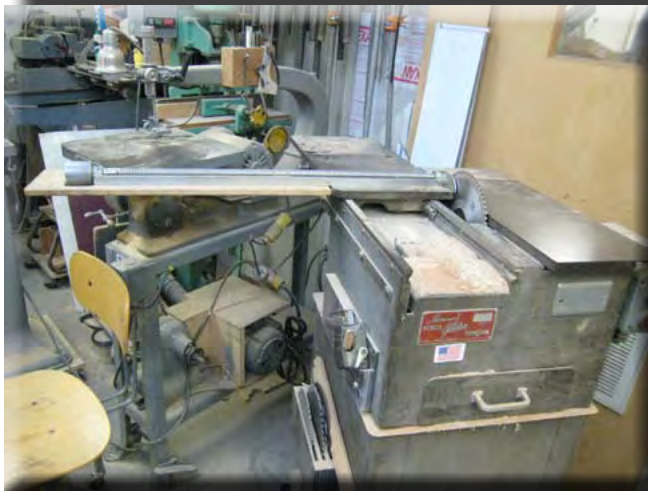
A Hammond Glider Line-a-Type printer's saw makes very accurate cuts. Is this a segmented turner's dream saw?
