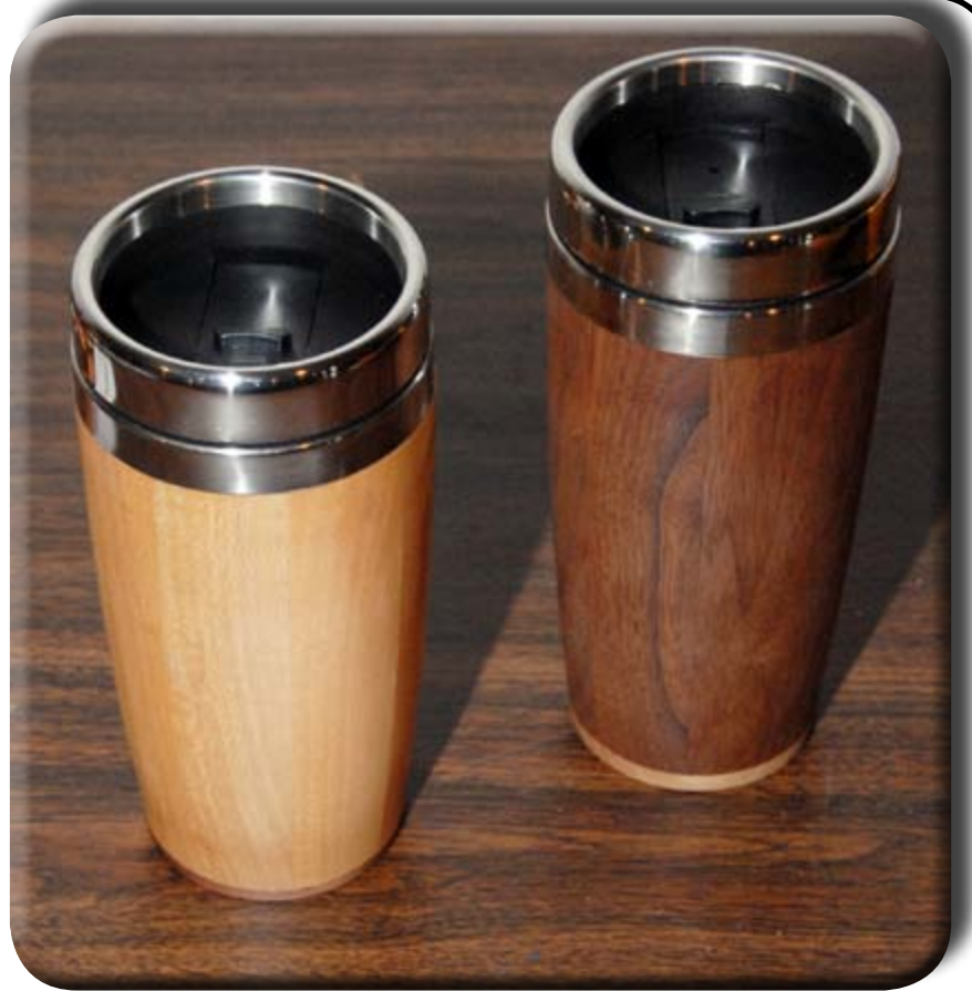
Peter Welch - showed his Sycamore stave construction coffee mug with a stainless liner and a Sycamore bottom and another turned from a single piece of Sycamore with a Walnut bottom.
