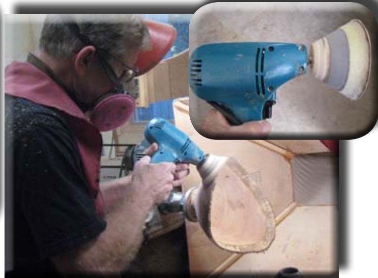
Fred sands without spinning it on the lathe, or sands while bowl is in his lap.
