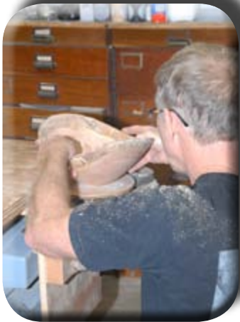
Bowl bottoms are flattened on a shop-made disc sander.
