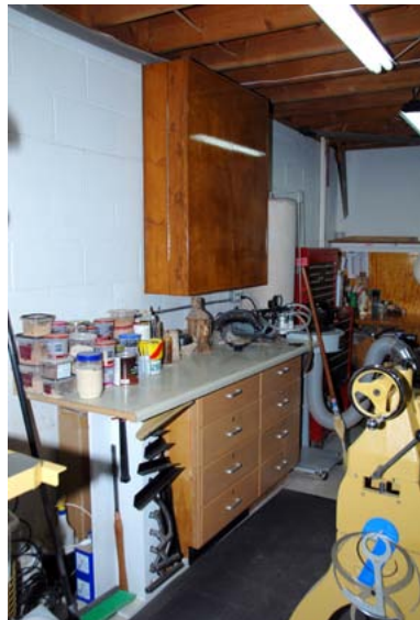
A 1960s walnut stereo cabinet was converted to an attractive storage and display cabinet for small turned pieces by removing the legs, radio receiver, turntable and speakers and then mounting it on a wall above book shelving. Woven reed panels in front of the speakers were removed and made into doors by adding hinges and turning knobs.
