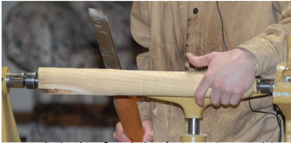
Nate made the chips fly with the Alan Lacer skew. He did briefly get some chatter and a spiral cut, which shows up in the photo above. That hard mulberry wood makes a great handle, but it can be a challenge to cut.
