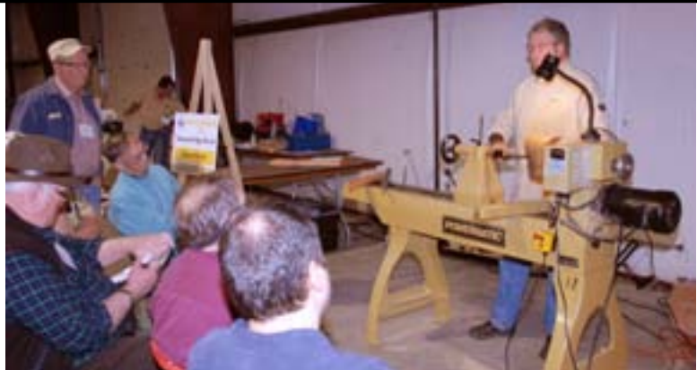
Peter Welch demonstrated the turning of natural edge bowls, and what can happen when turning a piece with a crack.
