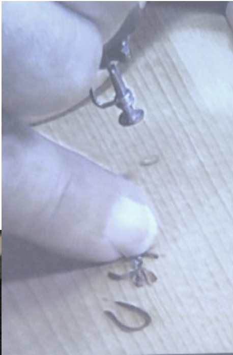
A brass/ copper thumb tack can be used to make a wood burning tip.
