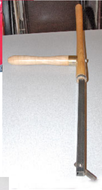
Jim Oates presented a hollow vessel turning tool from square tube with ash handle from a shovel and a shallow leaf-carved maple bowl.
