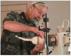
Since the handle has some flexibility to it, he was able to attach one end of Duct Tape to the tip and the other to the base of the hollow shape near the chuck to pull it back a bit to allow him to continue his hollowing. Don't forget, though, to check that tape occasionally, since if it slips, watch out! By the way, Tom insisted that he always uses the professional silver Duct Tape and never the sissy colored stuff. Makes all the difference.
