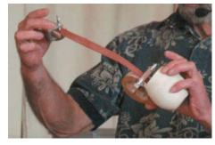
Although we had a slight break in the handle the first time through, Tom glued it and used a novel "sandwich" of wax paper on each side to contain the glue in the break. He then immersed the wood into the boiling water a second time to regenerate the wood's plastic
