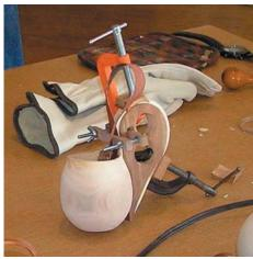
Item clamped and drying. The back strap has been released in this image.
