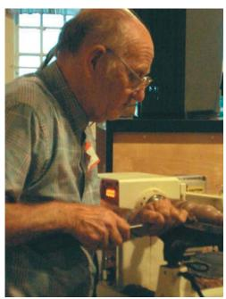
Miles illustrates his cutting techniques. He likes the gouge chisel, parting tool, and straight edge skew chisel. He uses a 5/16" and 3/8" drill at the top for the socket.
