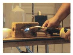
Ron heats the metal using a soft fire brick and a torch, watching for color change. He heats it twice to prepare the metal. First the metal is heated to a red hot color and after a quick cooling in water he heats it a second time, watching carefully to the color of sand.
