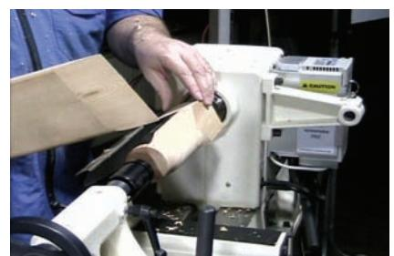
He does use the pointed (toe) end at times, to initiate those defining lines or the notches between beads, and maybe to make the final shearing cut across the end grain, but he highlighted the necessity to stay "one minute past or before midnight" with the trailing edge (depending on whether cutting on the left or right side) to avoid that deadly catch.
