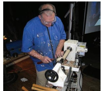
Here he is making those light cuts with the skew, leading with the blunt angle (heel) side.
