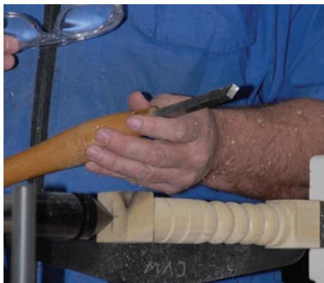
Willie next illustrated the Bedan tool. This 3/8" flat topped cutter has tapered sides, so that the bottom is narrower than the top. It was highly effective as certain cuts, such as the rounding over of beads in this photo.
