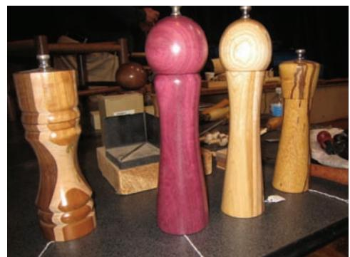
Turning these began with parting off the top third for the top and involved multiple mountings to achieve four different diameter drillings. The demo was slightly slowed by the lack of a key for the manual chuck he had along. His keyless chuck of choice would not fit our Jet. But he persevered and pulled it off fine. Using a careful final cut he is able to reduce the sanding necessary. Willie said sanding is the main reason he does not do bowls.
