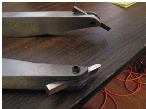
Here is a close-up of the single set screw that locks the bit in place at any angle.
