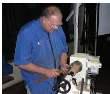
Although he uses the skew a good bit, he uses an inch and a half roughing gouge round off the corners, rotating the leading edge of the gouge with fluid movements left to right according to direction of cut, and always taking light cuts.
