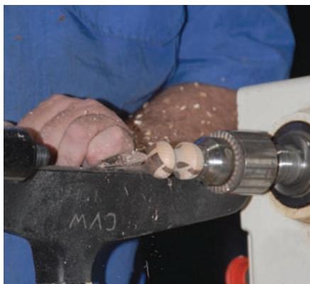
A spindle gouge with a steep fingernail grind can also be used to form beads or round over ends of knobs.
