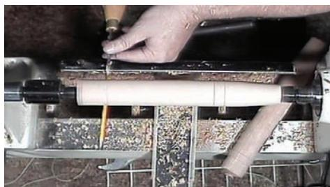
When turning the posts he makes pairs of lightly scribed lines with the skew spaced 3/4" apart. These are done by eye on the first leg and then copied to the following of the set. The lines will locate the centers of the rung holes, and are spaced so that the second rung tenon will overlap and cut into the one above or below it, locking them together.
