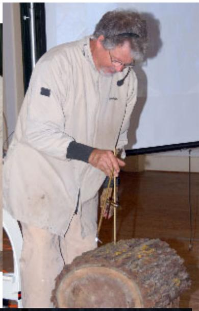
Giant calipers were used for layout.
