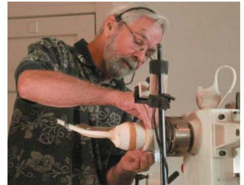
Since the handle has some flexibility to it, he was able to attach one end of Duct Tape to the tip and the other to the base of the hollow shape near the chuck to pull it back a bit to allow him to continue his hollowing. Don't forget, though, to check that tape occasionally, since if it slips, watch out! By the way, Tom insisted that he always uses the professional silver Duct Tape and never the sissy colored stuff. Makes all the difference.
