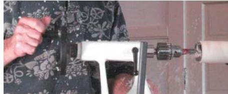
Although he laughed about not always having a plan, he stressed the importance of studying the grain closely before selecting which part of the flange to keep for his handle or handles (smart idea is to have two handles in case one breaks!). To achieve the strongest handles that will bend best without breaking, go with the grain, not against it. Look for quarter-sawn cut "faced grain" in comparison with "tangential faced" grain.
