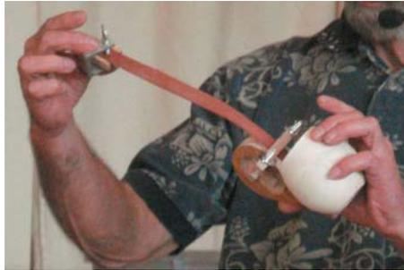
Although we had a slight break in the handle the first time through, Tom glued it and used a novel "sandwich" of wax paper on each side to contain the glue in the break. He then immersed the wood into the boiling water a second time to regenerate the wood's plastic qualities.
