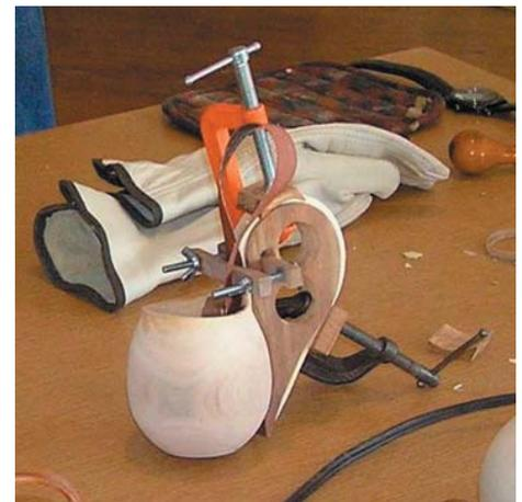
*Item clamped and drying. The back strap has been released in this image.*
