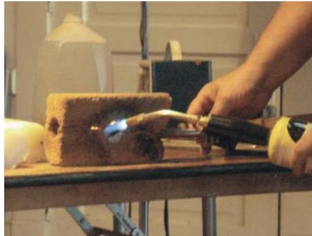
Ron heats the metal using a soft fire brick and a torch, watching for color change. He heats it twice to prepare the metal. First the metal is heated to a red hot color and after a quick cooling in water he heats it a second time, watching carefully to the color of sand.
