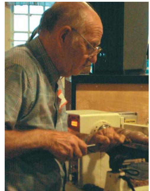
*Miles illustrates his cutting techniques. He likes the gouge chisel, parting tool, and straight edge skew chisel. He uses a 5/16" and 3/8" drill at the top for the socket.*
