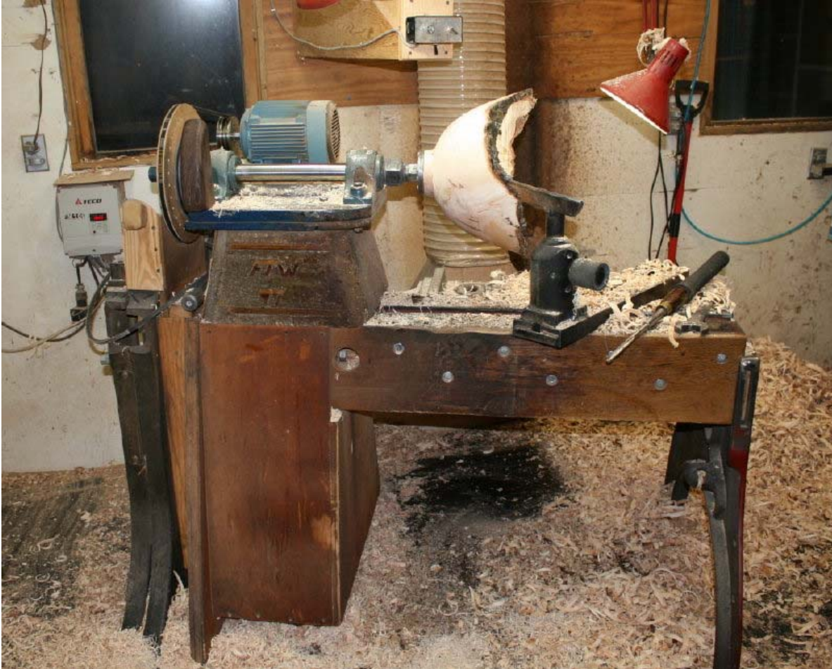
Here is a general view of the lathe. The bolt holes along the side attach the metal ways I added last year.
