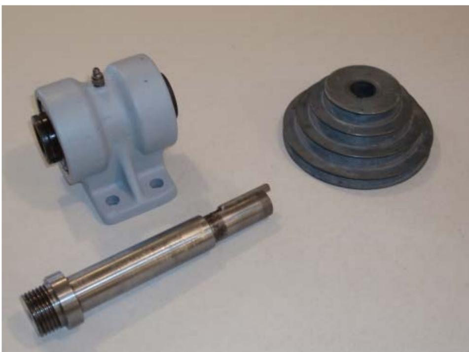
Because of the limited funds I mention earlier I started scrounging for parts at scrap metal dealers. I found the pillar block shown in the photo and some bar stock to use for the spindle.
