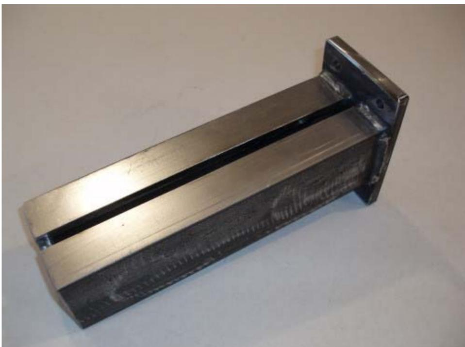
The lathe bed is made of 3" X 3" X 3/8" steel angle. The angle is welded to a 1/2" plate that will be bolted to the main post. There are several sets of holes drilled in the post so the bed can be moved up or down based on the diameter of the bowl to be turned.
