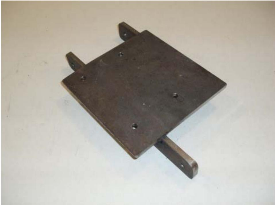
The motor mount is made of 1/4" flat steel plate welded to 1/4" flat bar stock. The motor mount will be bolted to the main post.
