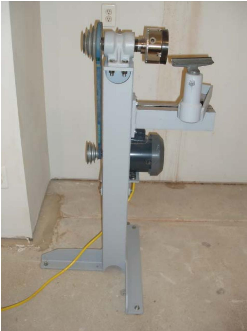
This photo shows the finished lathe with the exception of adding the switch. It has a 1 horsepower motor with a speed range of approximately 575 - 2300 RPM.
