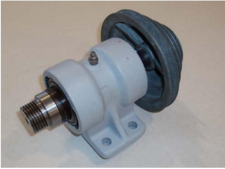
The completed spindle assembly.
