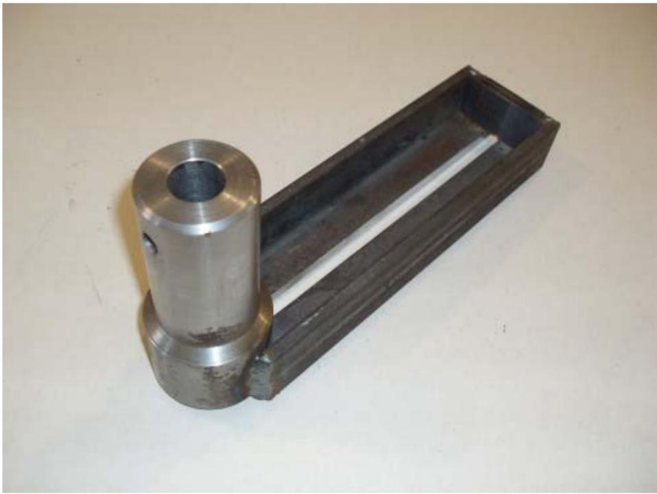
The banjo is made of 2" X 2" X 3/8" steel angle and a piece of 3" bar stock with the upper portion turned down to 2" diameter with a 1" hole for the tool rests.
