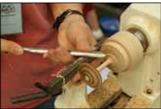
Alternative chucking method — turning block glued to waste wood which is attached to the faceplate
